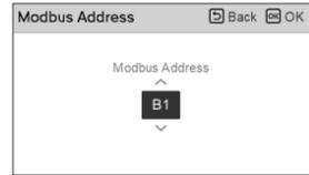
There are 2 options, modbus address and unit, in this function. Activating the modbus address option, you choose one address(B0 or B1) or don't use. Then, you set the port and specification in range of 0000.0~9999.9[pulse/kWh] as shown in the figure below.
