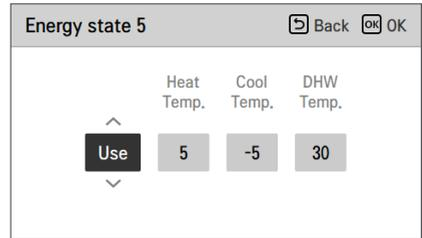
When Signal Mode of EES use type is selected, press the Digital Input Assignment button to set the energy state according to the input signal.
