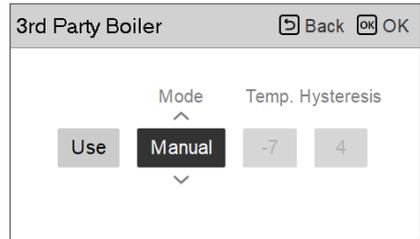
If the mode of this function is set to "Auto", you can set temperature of the boiler and hysteresis, respectively.
