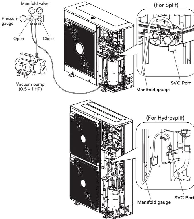
When selecting a vacuum, you should select one which is capable of achieving 0.2 Torr of ultimate vacuum. Degree of vacuum is expressed in Torr, micron, mmHg, and Pascal (Pa). The units correlate as follows:
