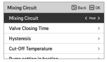
You can set valve closing time[s] and hysteresis temperature[°C] on screen by yourself. Setting the cut-off temperature protects the water from flowing over the cut-off temperature in the mixing circuit during heating operation.
