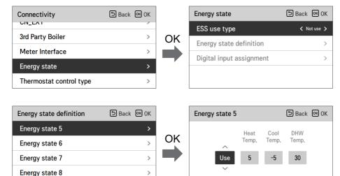
When Signal Mode of EES use type is selected, press the Digital Input Assignment button to set the energy state according to the input signal.
