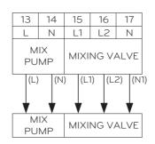
(L): Live signal from PCB to mix pump
