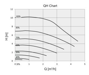
Performance test based on standard ISO 9906 with pre-pressure 2.0bar and liquid temperature 20 °C.
