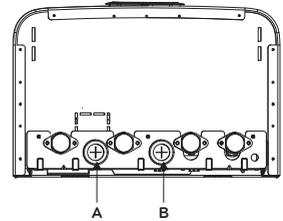
Hole A : For DC line (wire which is connected to the PCB of the control box)
