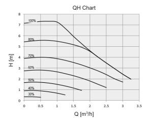
MGQ62321901: UPML GEO 20-105 CHBL (12 kW, 14 kW, 16 kW / For Split R410A Indoor unit 5 Series, For Hydrosplit)
