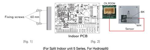
Step 6. Integrate the remote temperature sensor with the screws as the order of arrows.
