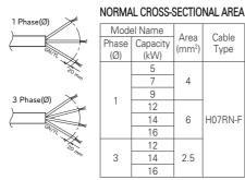
The connecting cable connected to the outdoor unit should be complied with IEC 60245 or HD 22.4 S4 (This equipment shall be provided with a cord set complying with the national regulation.)
