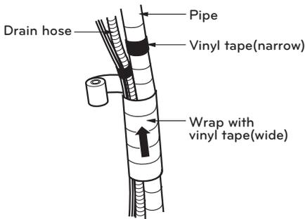
Do pipe forming by wrapping the connecting cable and refrigerant pipe (between the indoor unit and outdoor unit) with thermal insulation material and secure it with two kinds of vinyl tape.
