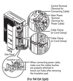
**Step 3.**: Use cable clamps (or cord clamps) to prevent unintended move of Power cable and Connecting cable.
