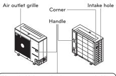
Always hold the unit by the corners, as holding it by the side intake holes on the casing may cause them to deform.
