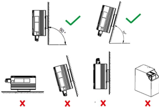
Inverters should be in a vertical position, a 50° backwards tilt is permitted.
