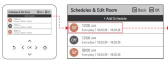
You can check the set timer's operation information (operation On/Off, operation mode, desired temperature), timer time, period, and day of week.
