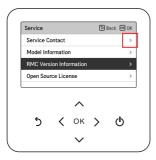
In each detail screen of the menu, as in the box in the left figure, if only ">" icon is displayed, you can move to the detail setting screen by pressing [>(right) or OK] button.
