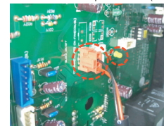
Transmission connector & LED in inverter compressor PCB
