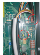
Transmission connector & LED in MAIN PCB
