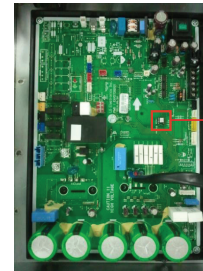
Correct insertion direction of inverter EEPROM
