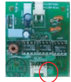
Indoor unit communication PCB
