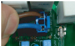
Inverter PCB assembly power connection
